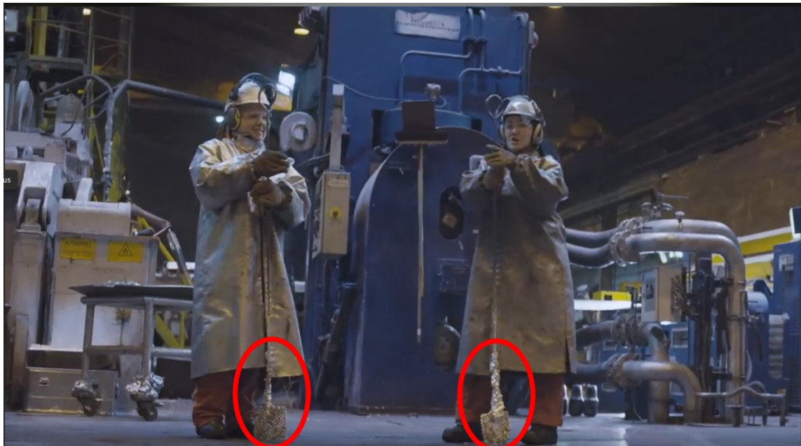
Figure 4. Hand tools covered with solidified aluminium.
